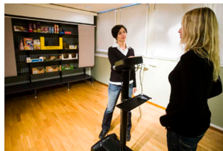
A respondent in front of a Tobii X120 Eye Tracker and a life-size store shelf projection.
