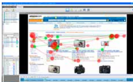
Gaze plots from two test subjects, trying to compare two digital cameras at an e-commerce website.
